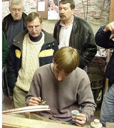
JIM MCDONALD REPAIRS PITS IN CHROME USING SILVER SOLDER
