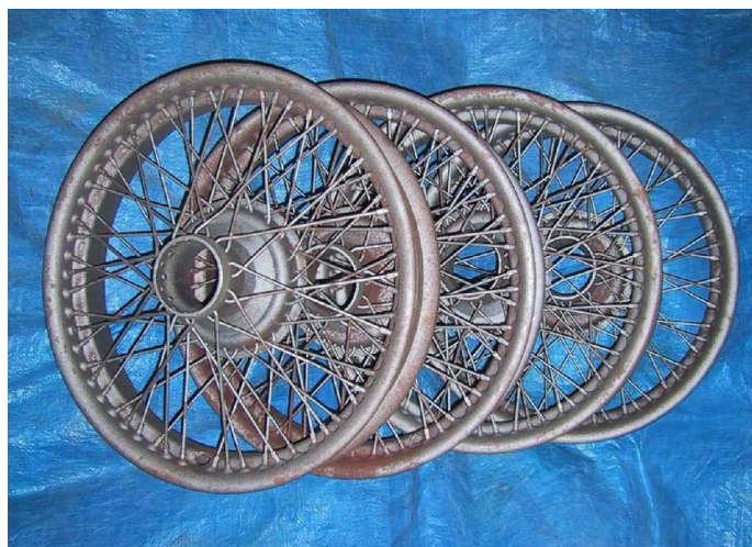
Rims cleaned by Wheelabrator process ready for rebuilding
